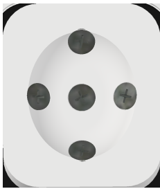
Fig. 3. Pin layout of the resistance based finger sensor.
