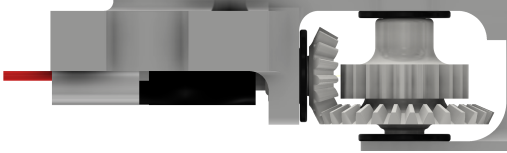
Fig. 2. Two part gearbox, the motor is connected to the left bevel gear.
